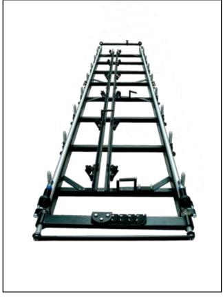
2.2.6.a. - Two tracks with cable carrier
