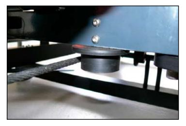
11. After finished shooting on track ensure that the end of the wire with eye-bold is always stored in it's holder. A sensor in the holder ensures that the track motor is switched off and that the wire drum in the bas can not be damaged.
