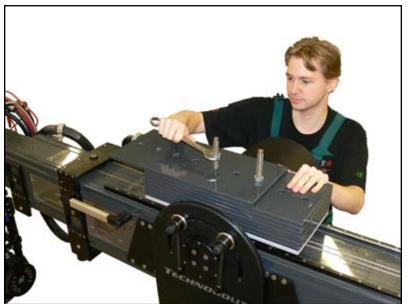
1.3. – Tightening a M24 hexagon nut onto counterweights
