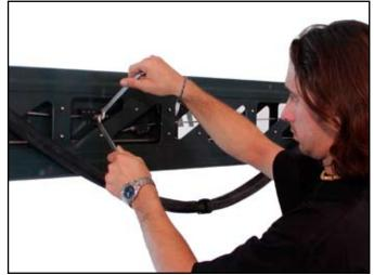
2.6.1.f – Securing nut with two spanners
