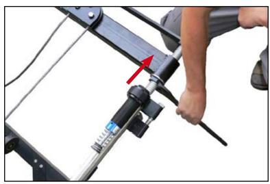
10. Tighten the wire until the big spring is not visible any more.
