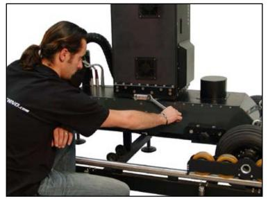
2.3.2.a. - Locking the crane pan brake by hand
