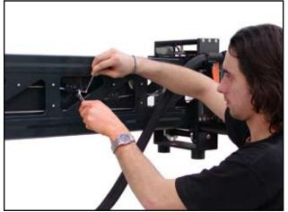
2.6.1.e – Tightening the cables
