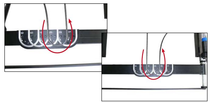
9. Tighten the wire with the use of the plastic nut.
