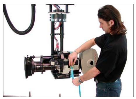
2.9.2.b - Securing the camera with a strap
