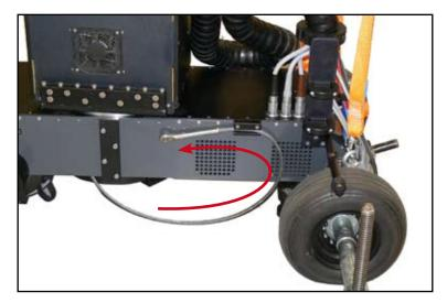
2. Attach the wire with the eye-bold to the end of the rail.
