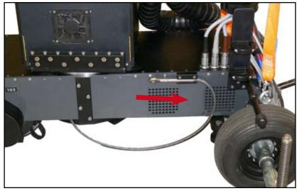
12. Restore the wire in the nest after shootin in order to avoid any damage to the wire.
