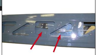
2.6.1.c - Anchorage pulling in and out cable (3rd beam section)
