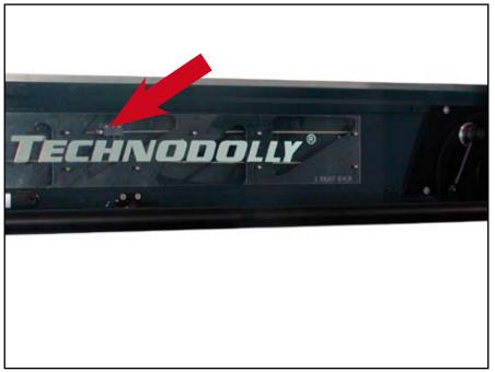
2.6.1.a - Anchorage pulling out cable (2nd beam section)
