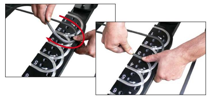
5. Lock the wire with the three clamping screws at the clamping plate.
