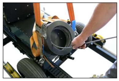
4. Lay the wire into the curved slot at the other end of the track. Pull the wire by hand as tight as possible.
