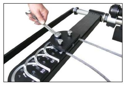
6. Take care that you use the correct slot. And take care that you insert the wire in the correct direction. If you use only one track insert the wire in slot no. 1 (take care of the reversed direction).
