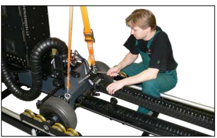
2.2.6.e. - Attaching the cable carrier to the base
