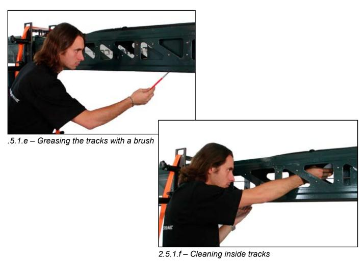
It is also important to clean the tracks on which the counterweight carriage rides on the first beam. These tracks carry a moving load of 200 kg (440 lbs.). Any dirt will cause slight vibrations that will be transferred to the film image.
