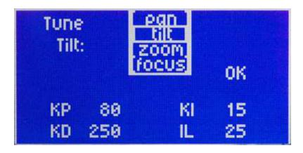
These settings are factory preset, and should never be changed. If they have been changed, they must be changed back to the following, or the Pan and Tilt motors can be damaged.
