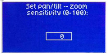
PT-Z can be adjusted between 0-100. The greater the number the slower the pan and tilt axes will respond according to the position of the zoom axis. When 0 is selected, zoom will not affect the pan and tilt axes.
